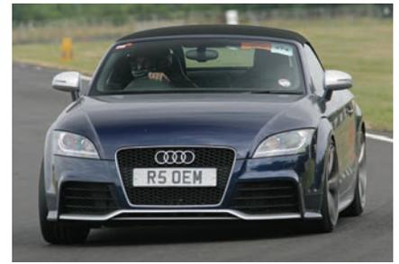
Track Pack is height-adjustable by 20 mm both front and rear, also providing the small degree of adjustment for accurate corner weighting.
